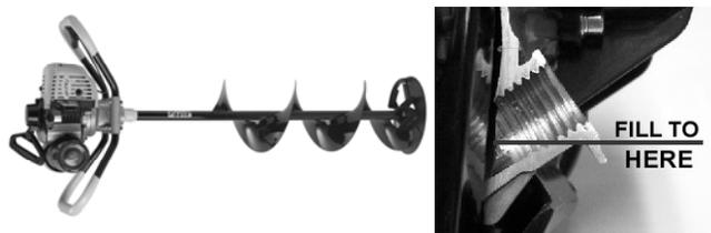
4. Turn oil-fill cap counter-clockwise and remove cap from oil-fill opening. Proper oil level should come to the middle of the threads in the lower part of the oil fill hole, as pictured above.
